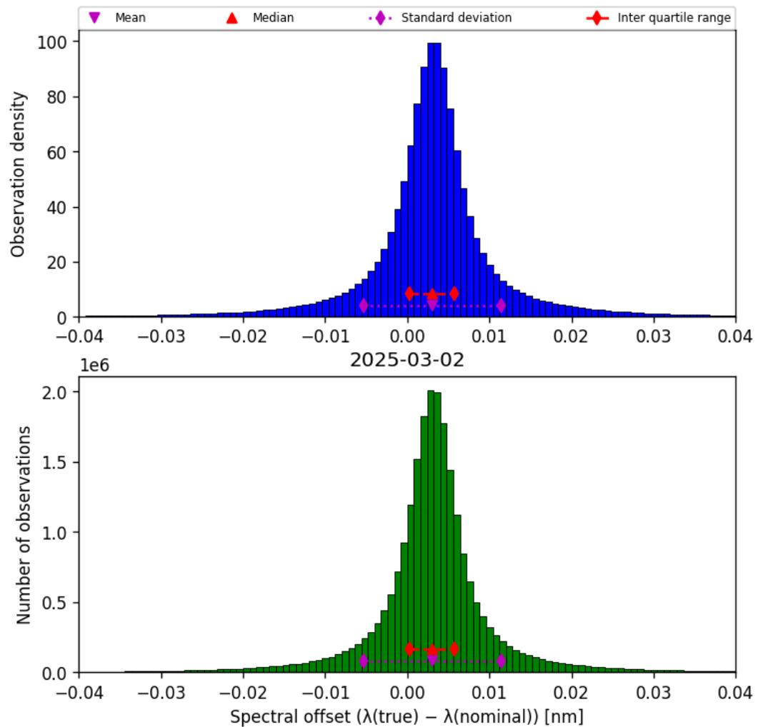
Figure 43: Histogram of “Spectral offset ( $\lambda_{\text{true}} - \lambda_{\text{nominal}}$ )” for 2025-03-02 to 2025-03-03
