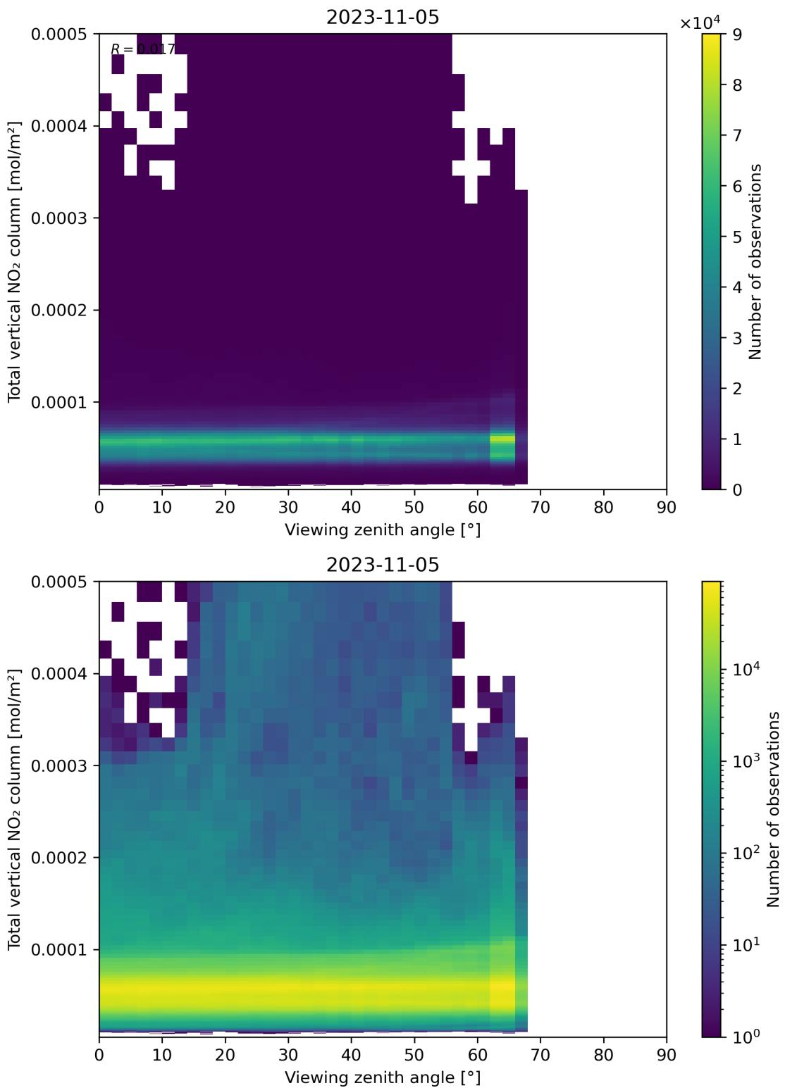
Figure 167: Scatter density plot of “Viewing zenith angle” against “Total vertical NO<sub>2</sub> column” for 2023-11-04 to 2023-11-06.
