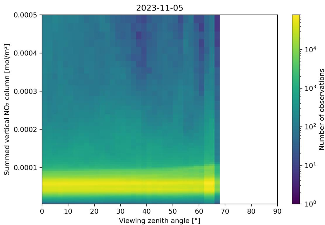
Figure 165: Scatter density plot of “Viewing zenith angle” against “Summed vertical NO<sub>2</sub> column” for 2023-11-04 to 2023-11-06.
