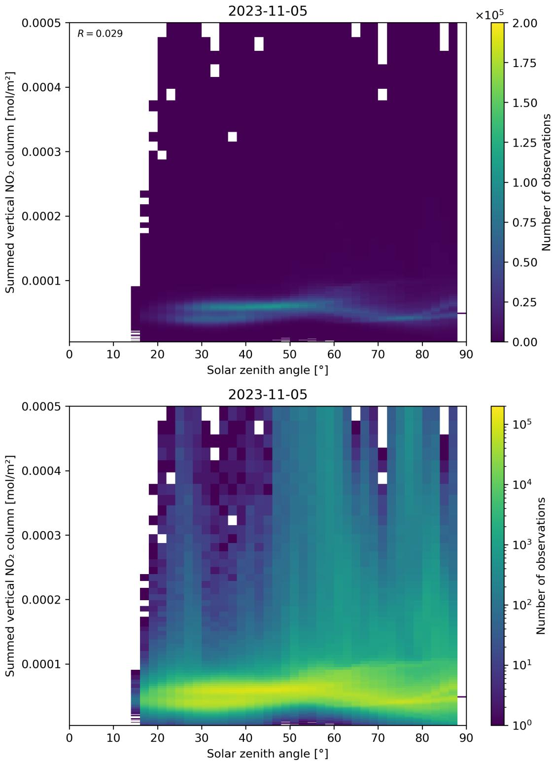
Figure 151: Scatter density plot of “Solar zenith angle” against “Summed vertical NO<sub>2</sub> column” for 2023-11-04 to 2023-11-06.
