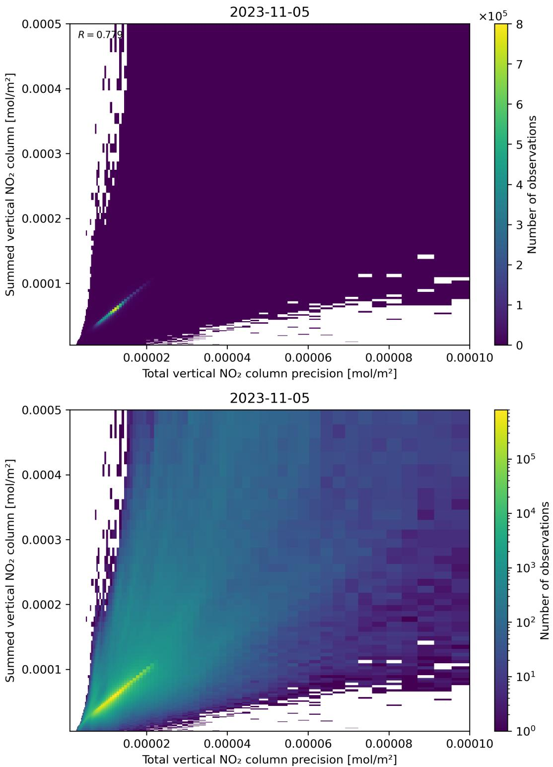
Figure 117: Scatter density plot of “Total vertical NO<sub>2</sub> column precision” against “Summed vertical NO<sub>2</sub> column” for 2023-11-04 to 2023-11-06.
