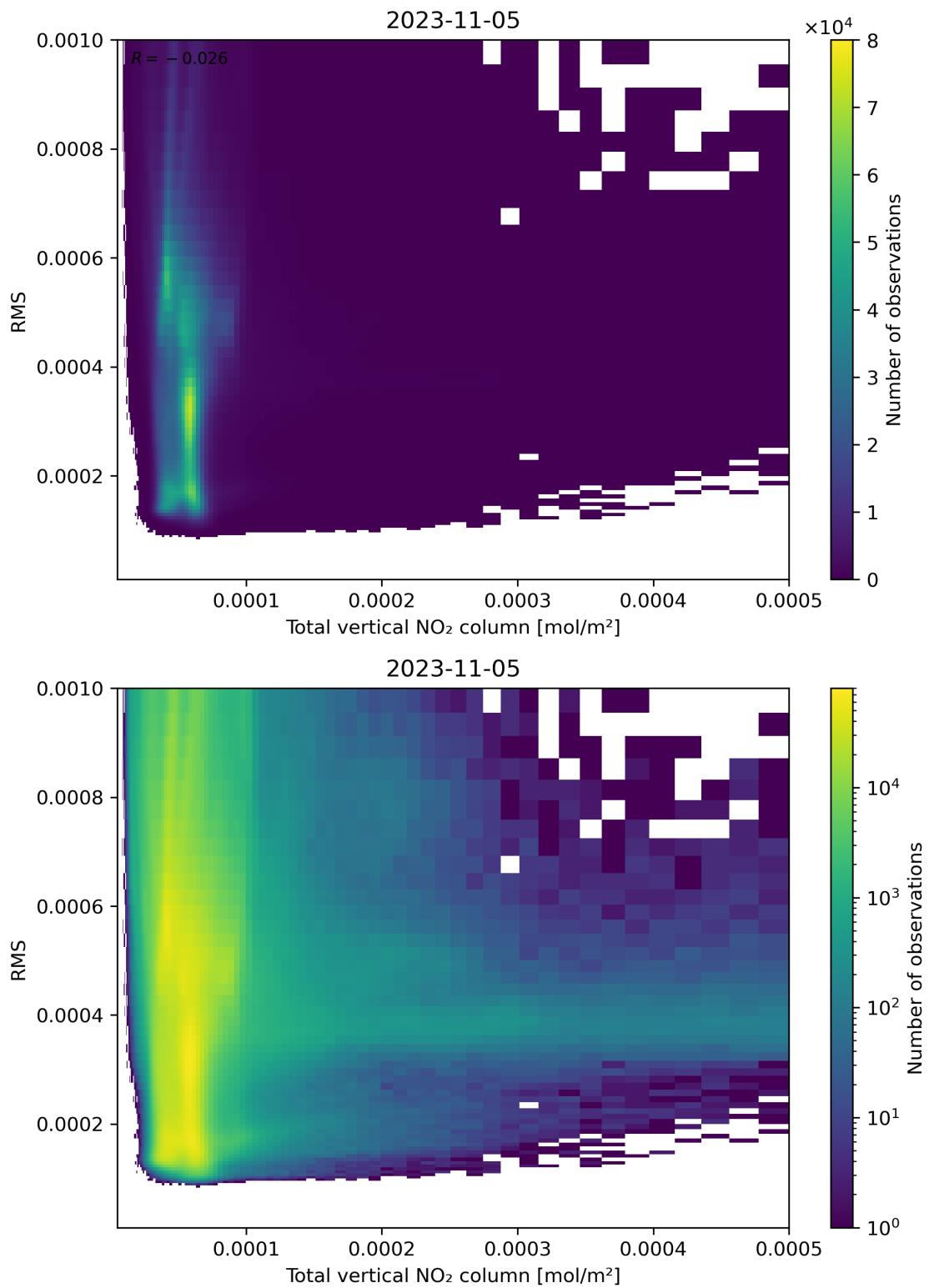
Figure 120: Scatter density plot of “Total vertical  $\text{NO}_2$  column” against “RMS” for 2023-11-04 to 2023-11-06.
