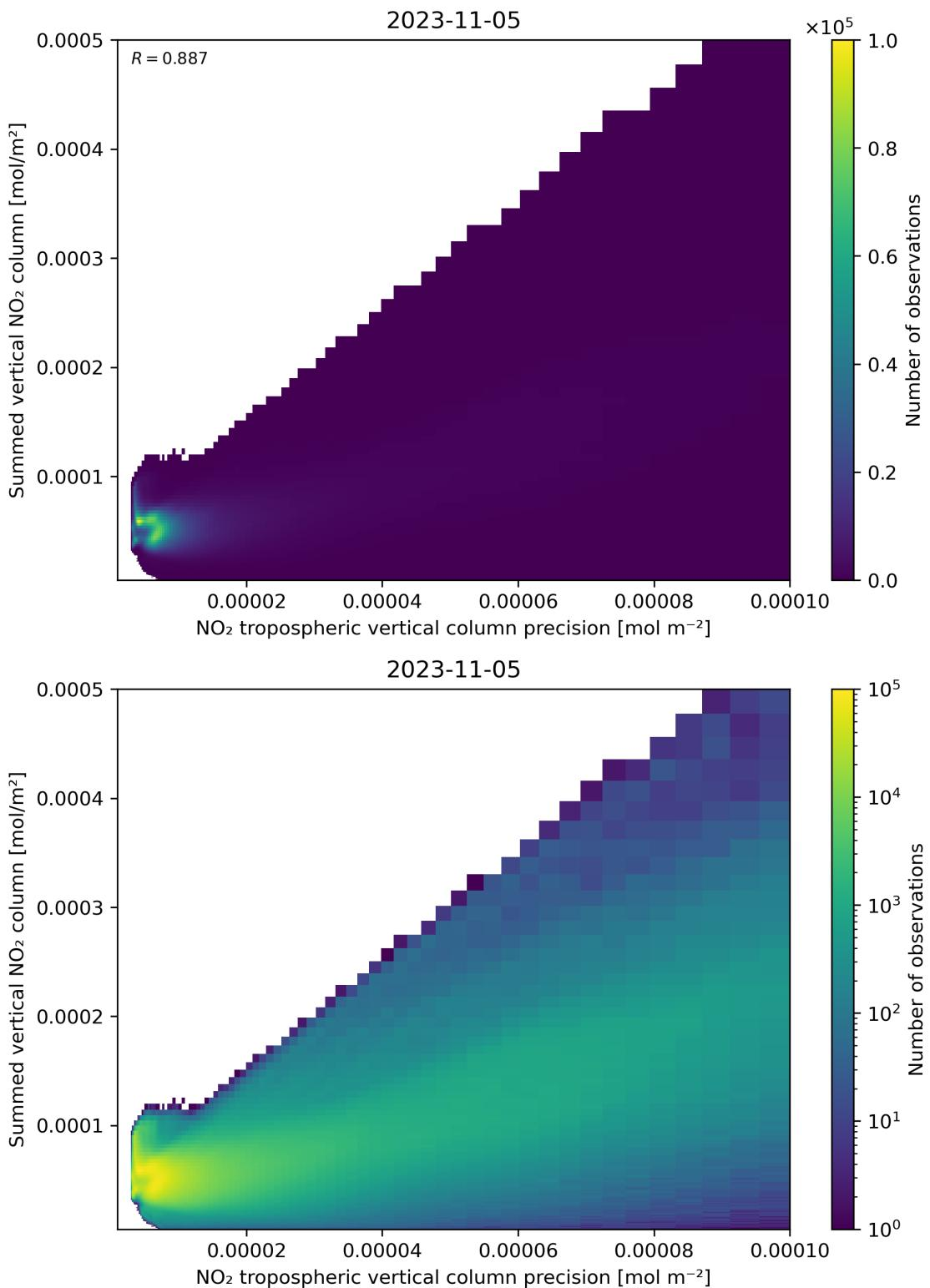
Figure 136: Scatter density plot of “NO<sub>2</sub> tropospheric vertical column precision” against “Summed vertical NO<sub>2</sub> column” for 2023-11-04 to 2023-11-06.
