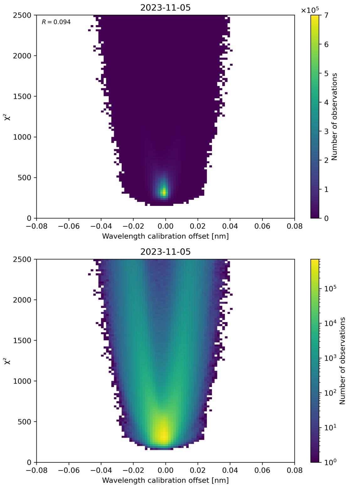
Figure 175: Scatter density plot of “Wavelength calibration offset” against “ $\chi^2$ ” for 2023-11-04 to 2023-11-06.
