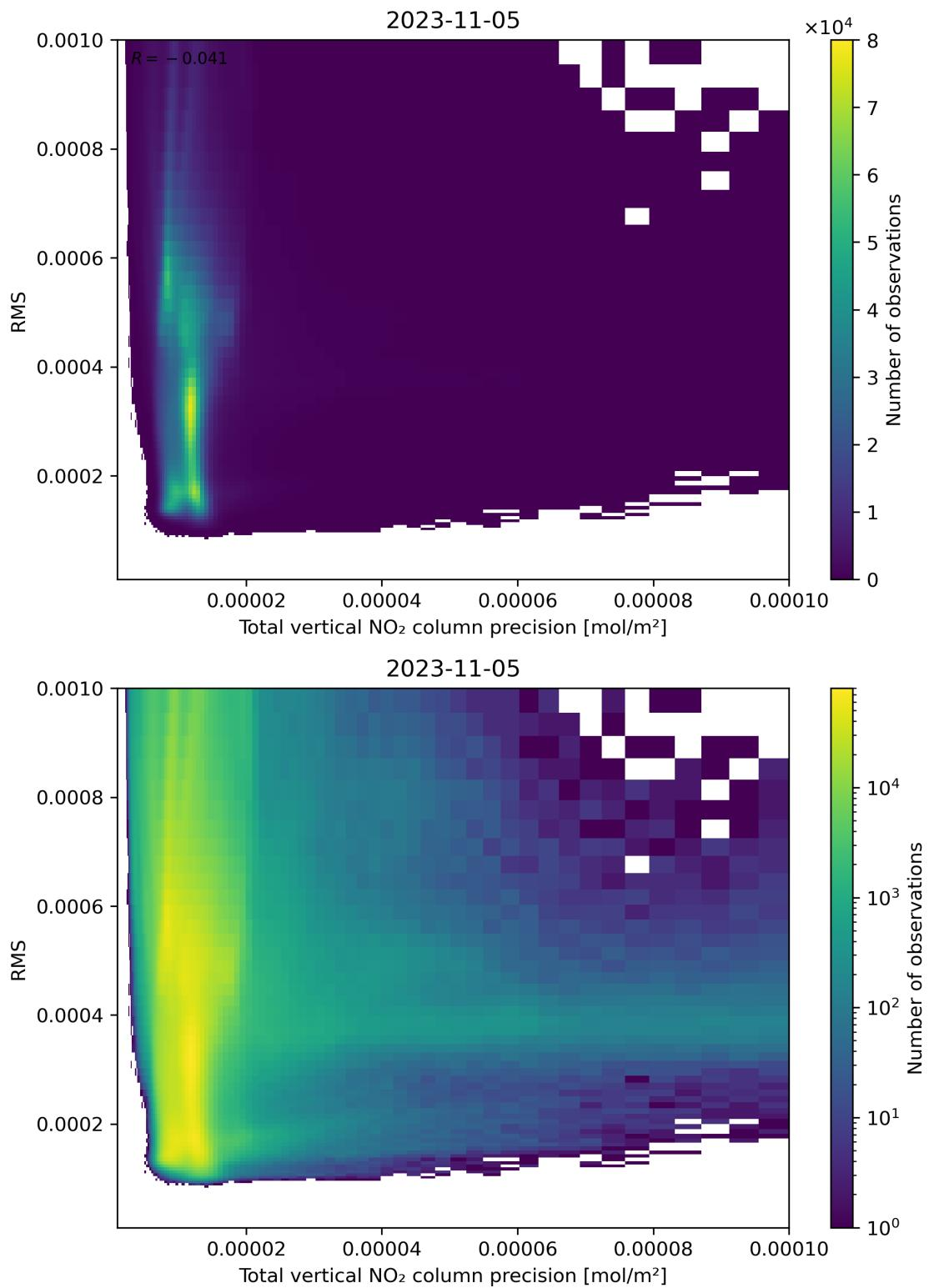
Figure 119: Scatter density plot of “Total vertical NO<sub>2</sub> column precision” against “RMS” for 2023-11-04 to 2023-11-06.
