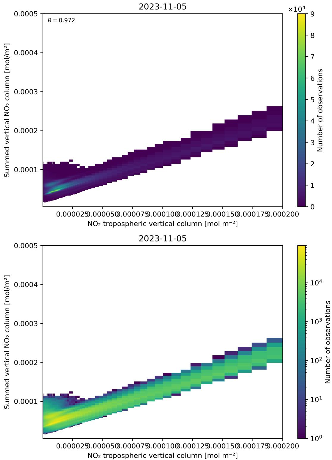
Figure 126: Scatter density plot of “NO<sub>2</sub> tropospheric vertical column” against “Summed vertical NO<sub>2</sub> column” for 2023-11-04 to 2023-11-06.
