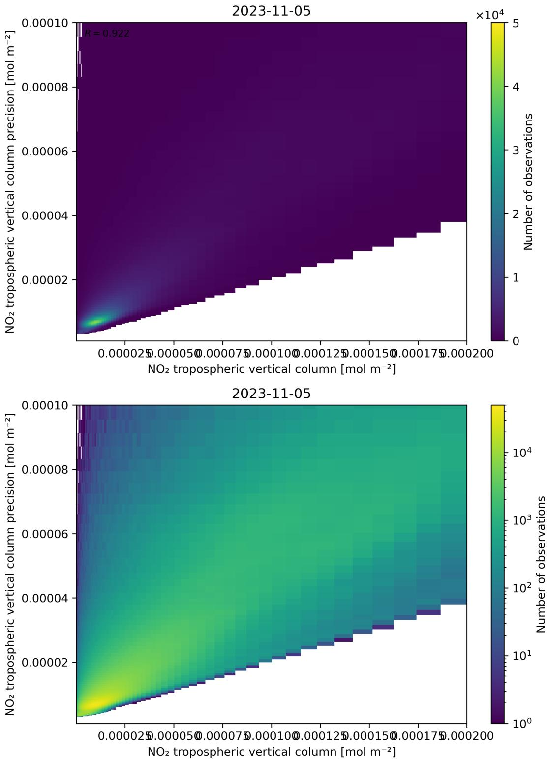
Figure 130: Scatter density plot of “NO<sub>2</sub> tropospheric vertical column” against “NO<sub>2</sub> tropospheric vertical column precision” for 2023-11-04 to 2023-11-06.
