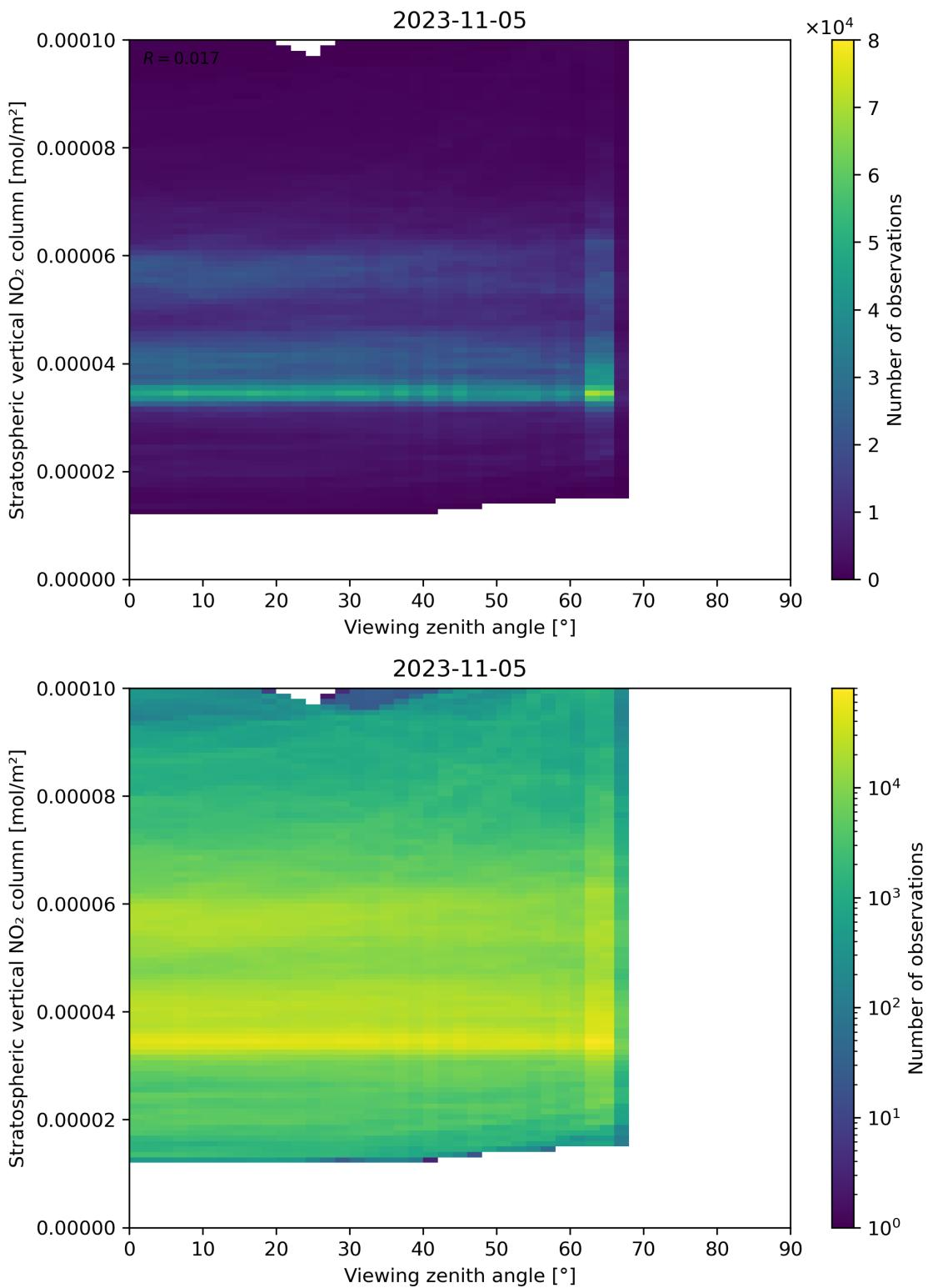
Figure 164: Scatter density plot of “Viewing zenith angle” against “Stratospheric vertical  $\text{NO}_2$  column” for 2023-11-04 to 2023-11-06.
