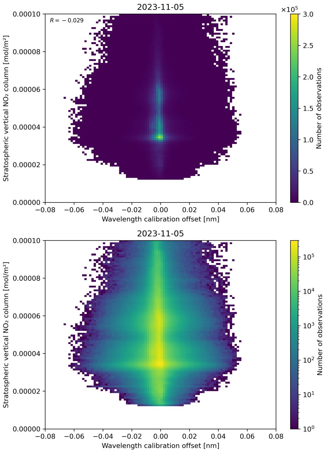
Figure 176: Scatter density plot of “Wavelength calibration offset” against “Stratospheric vertical NO<sub>2</sub> column” for 2023-11-04 to 2023-11-06.
