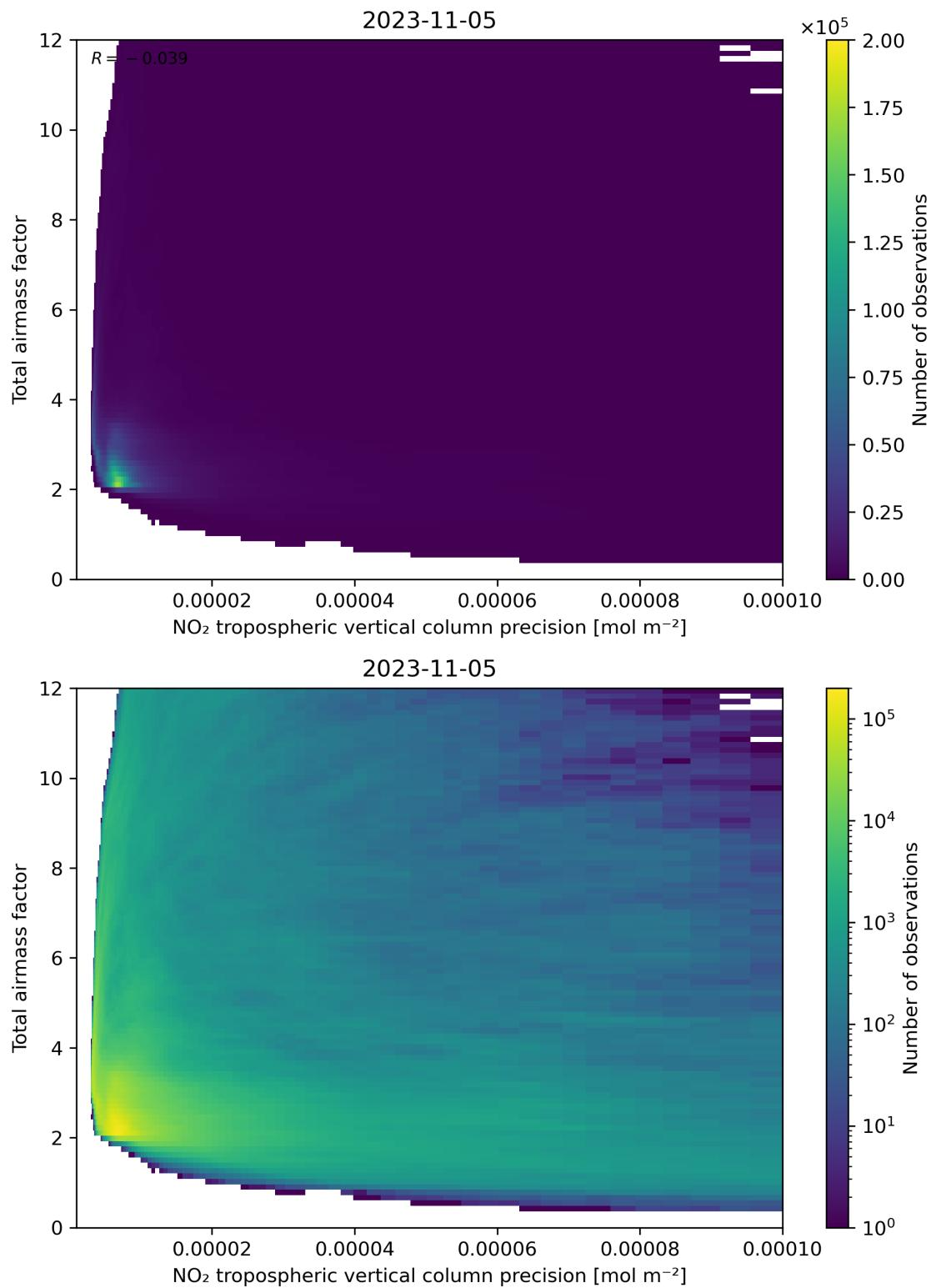
Figure 132: Scatter density plot of “NO<sub>2</sub> tropospheric vertical column precision” against “Total airmass factor” for 2023-11-04 to 2023-11-06.
