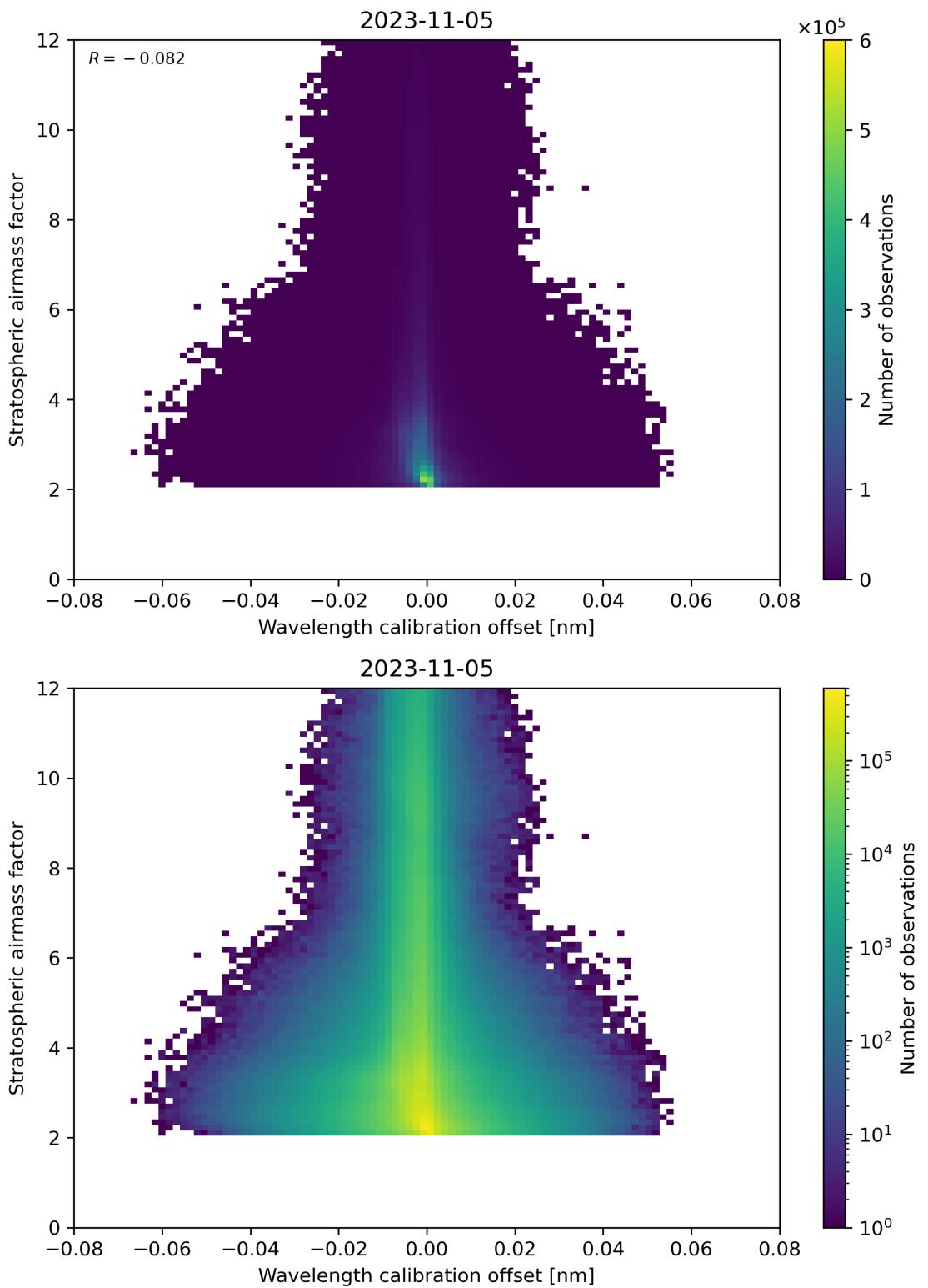
Figure 174: Scatter density plot of “Wavelength calibration offset” against “Stratospheric airmass factor” for 2023-11-04 to 2023-11-06.
