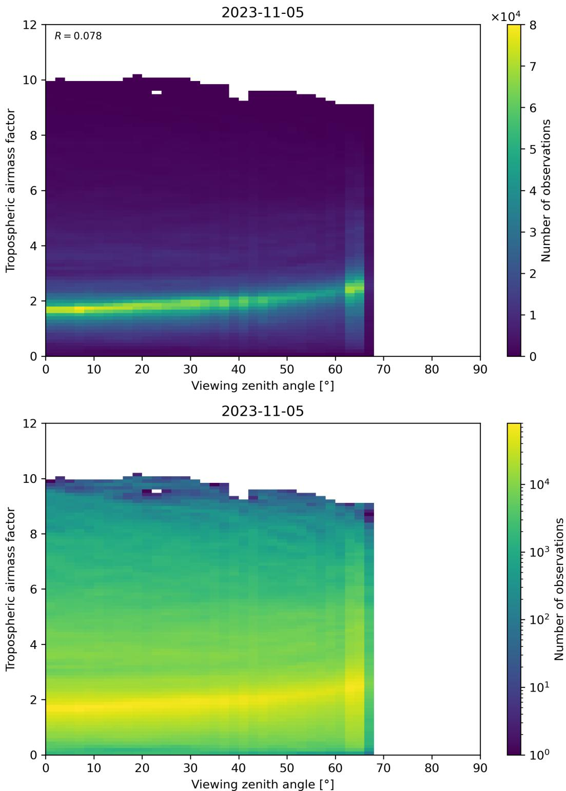
Figure 161: Scatter density plot of “Viewing zenith angle” against “Tropospheric airmass factor” for 2023-11-04 to 2023-11-06.
