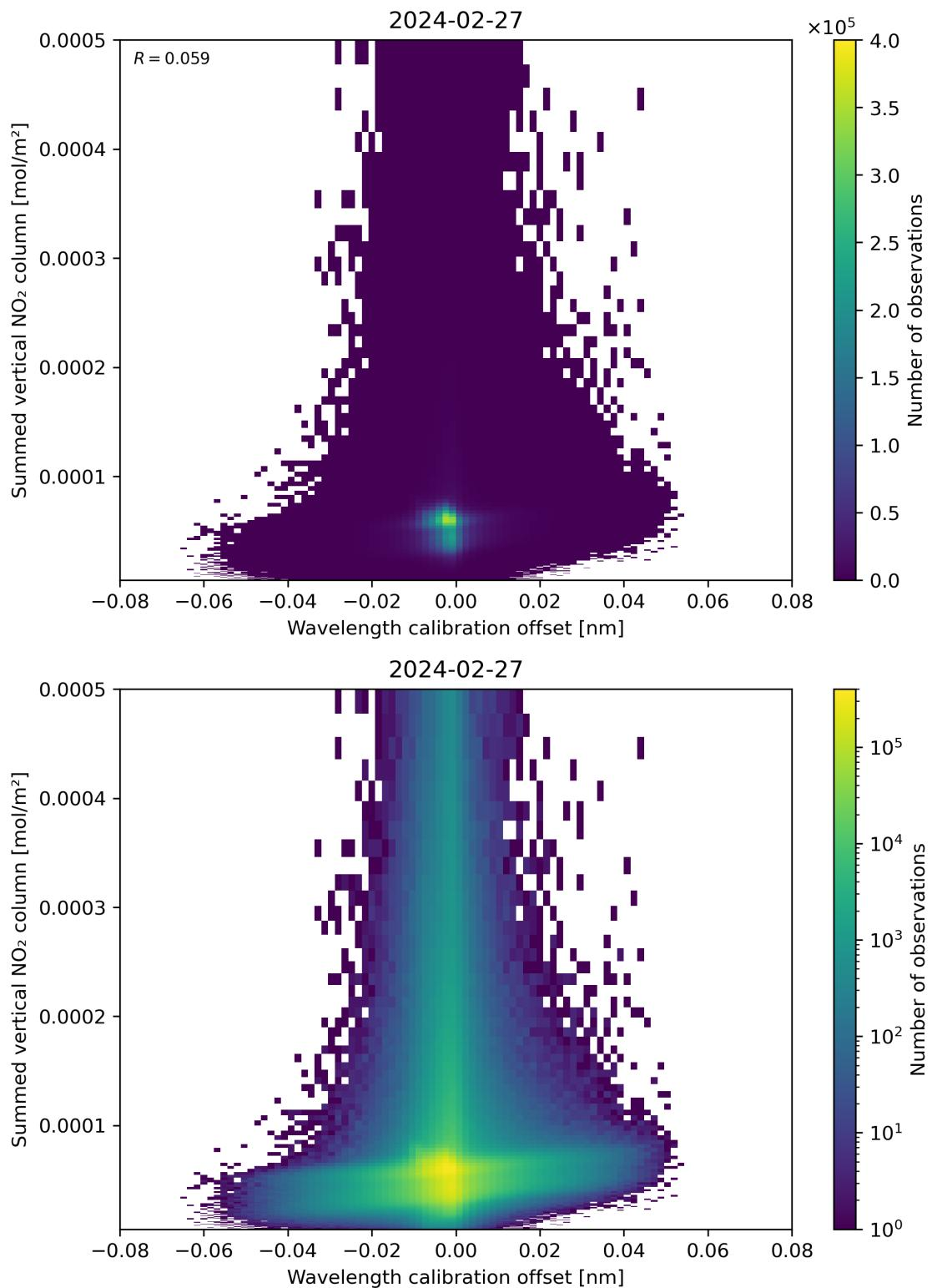
Figure 177: Scatter density plot of “Wavelength calibration offset” against “Summed vertical NO<sub>2</sub> column” for 2024-02-27 to 2024-02-28.
