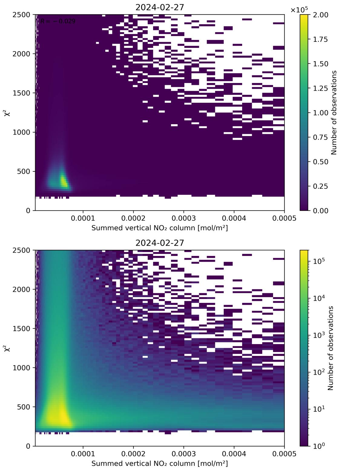
Figure 104: Scatter density plot of “Summed vertical NO<sub>2</sub> column” against “ $\chi^2$ ” for 2024-02-27 to 2024-02-28.
