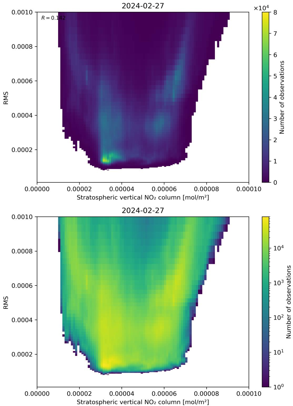
Figure 102: Scatter density plot of “Stratospheric vertical  $\text{NO}_2$  column” against “RMS” for 2024-02-27 to 2024-02-28.
