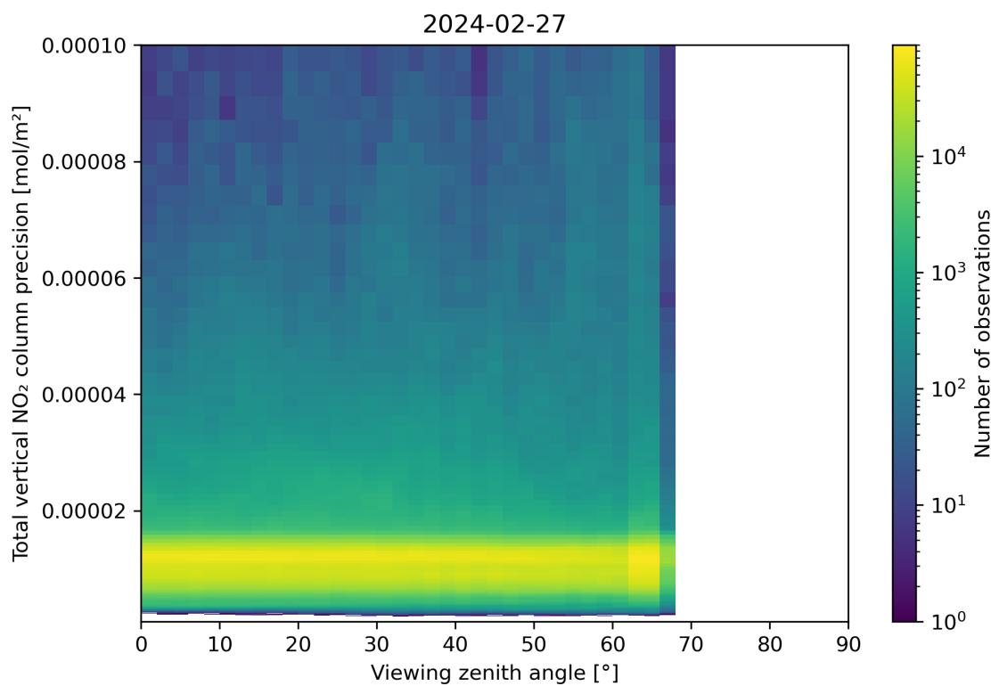
Figure 168: Scatter density plot of “Viewing zenith angle” against “Total vertical NO<sub>2</sub> column precision” for 2024-02-27 to 2024-02-28.
