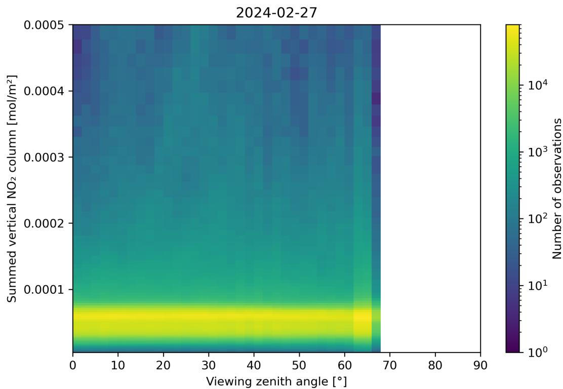
Figure 165: Scatter density plot of “Viewing zenith angle” against “Summed vertical NO<sub>2</sub> column” for 2024-02-27 to 2024-02-28.
