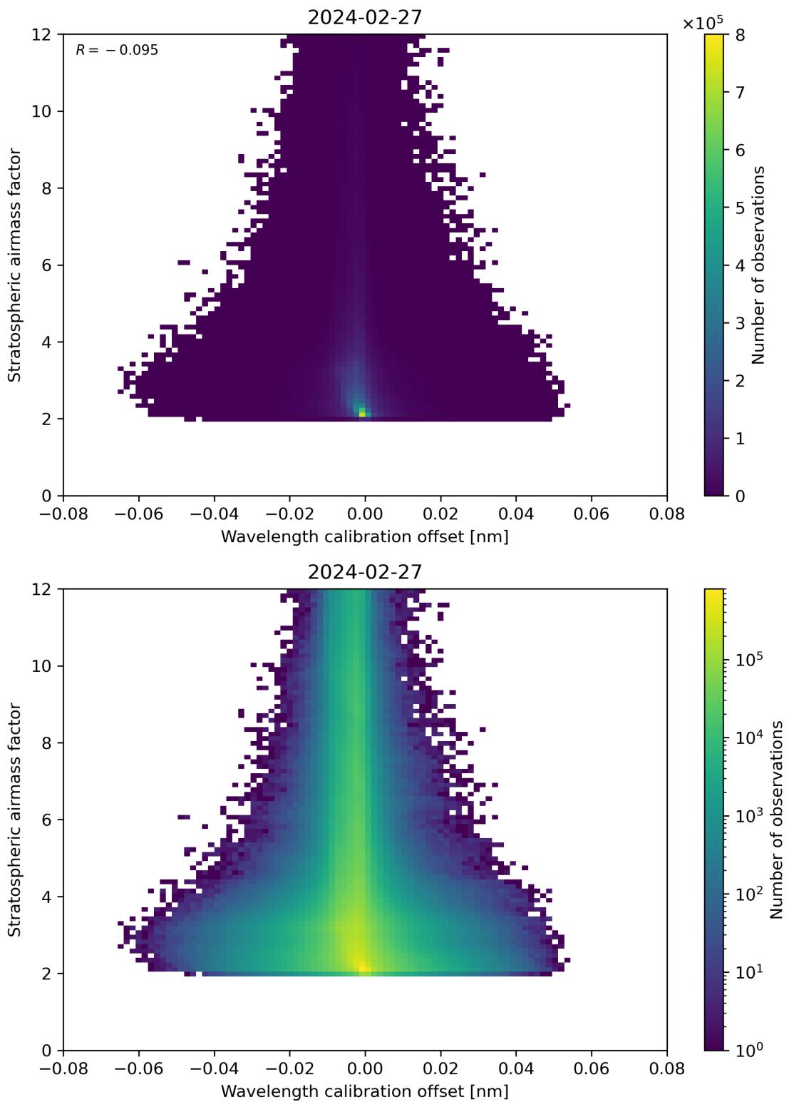
Figure 174: Scatter density plot of “Wavelength calibration offset” against “Stratospheric airmass factor” for 2024-02-27 to 2024-02-28.
