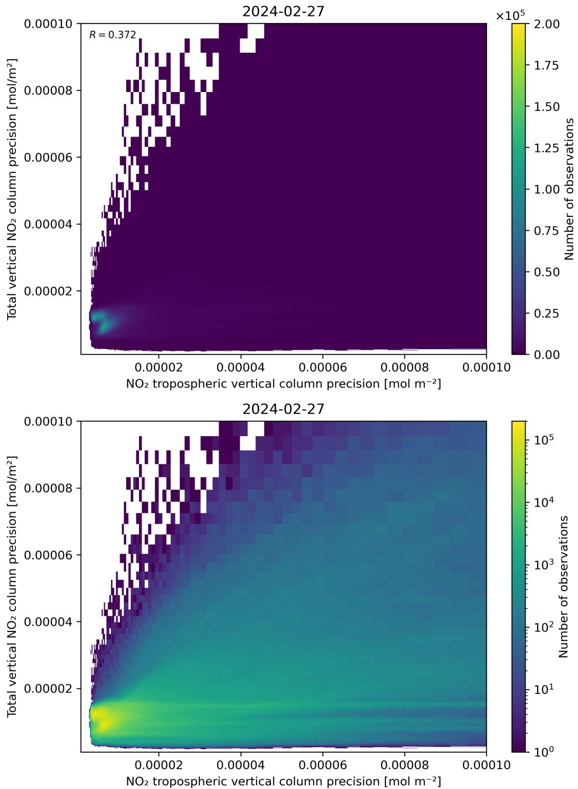
Figure 139: Scatter density plot of “NO<sub>2</sub> tropospheric vertical column precision” against “Total vertical NO<sub>2</sub> column precision” for 2024-02-27 to 2024-02-28.
