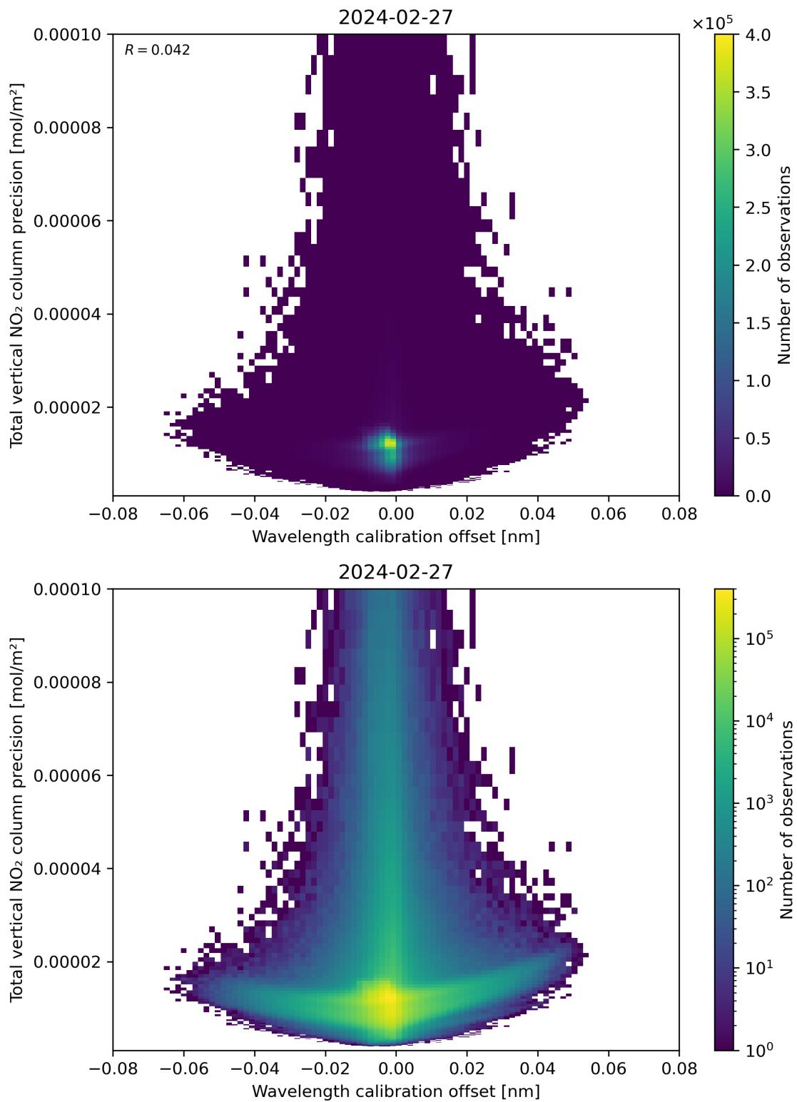
Figure 180: Scatter density plot of “Wavelength calibration offset” against “Total vertical  $\text{NO}_2$  column precision” for 2024-02-27 to 2024-02-28.
