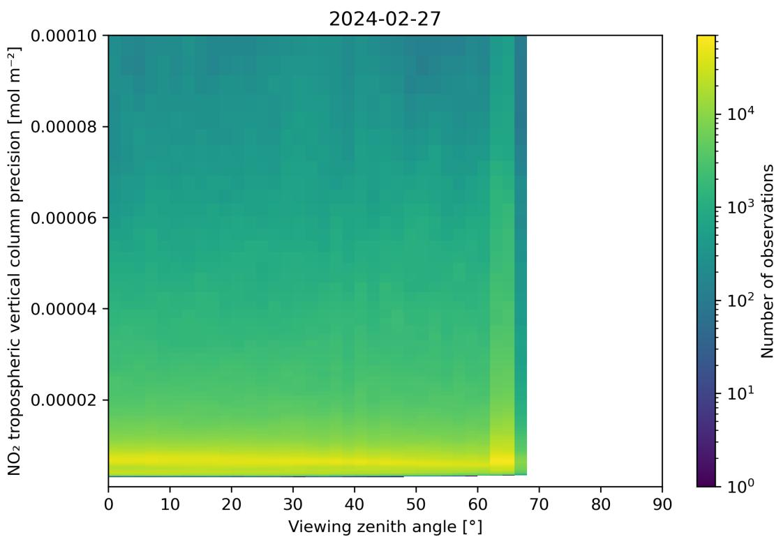
Figure 170: Scatter density plot of “Viewing zenith angle” against “ $\text{NO}_2$  tropospheric vertical column precision” for 2024-02-27 to 2024-02-28.
