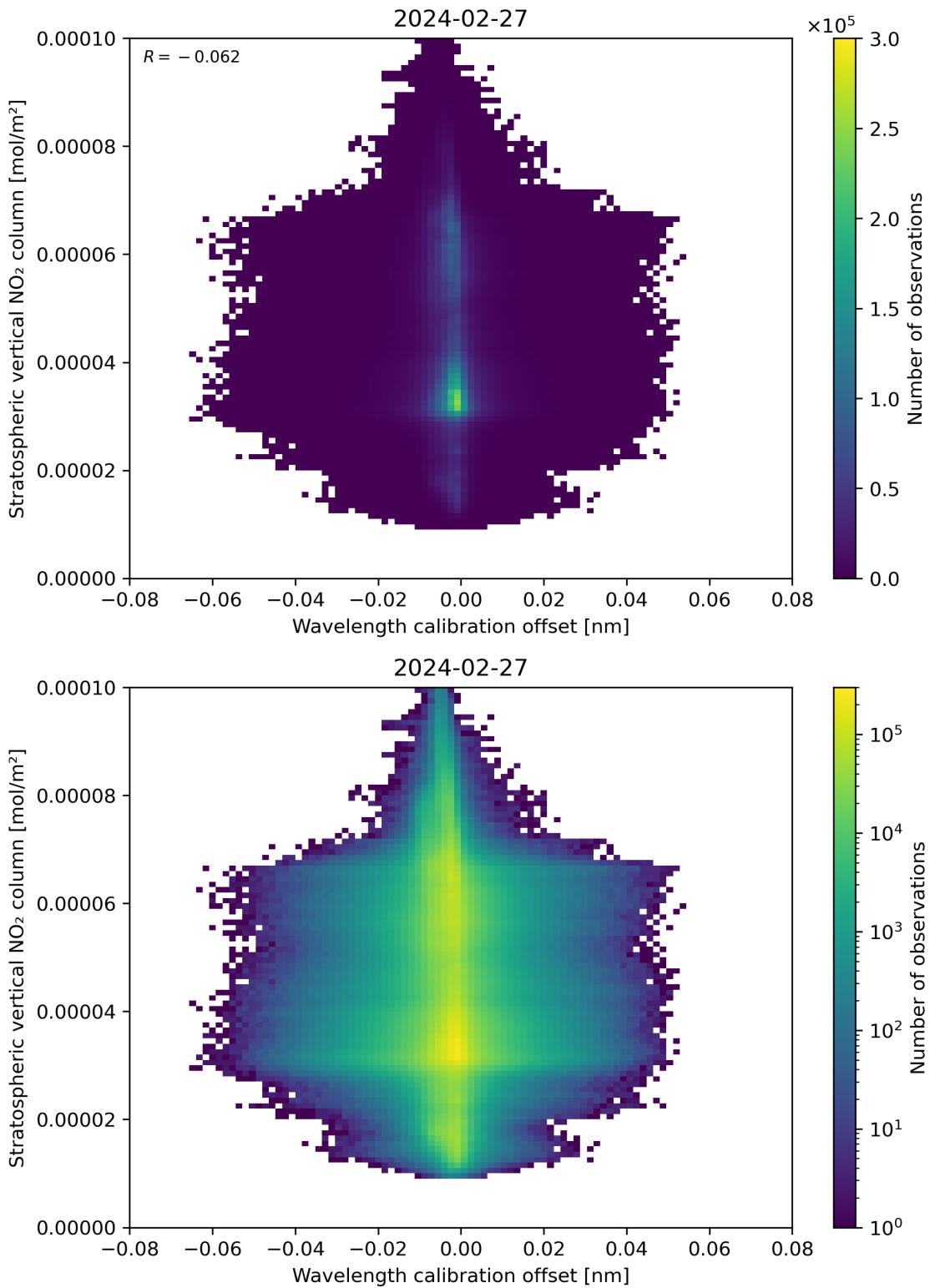
Figure 176: Scatter density plot of “Wavelength calibration offset” against “Stratospheric vertical NO<sub>2</sub> column” for 2024-02-27 to 2024-02-28.
