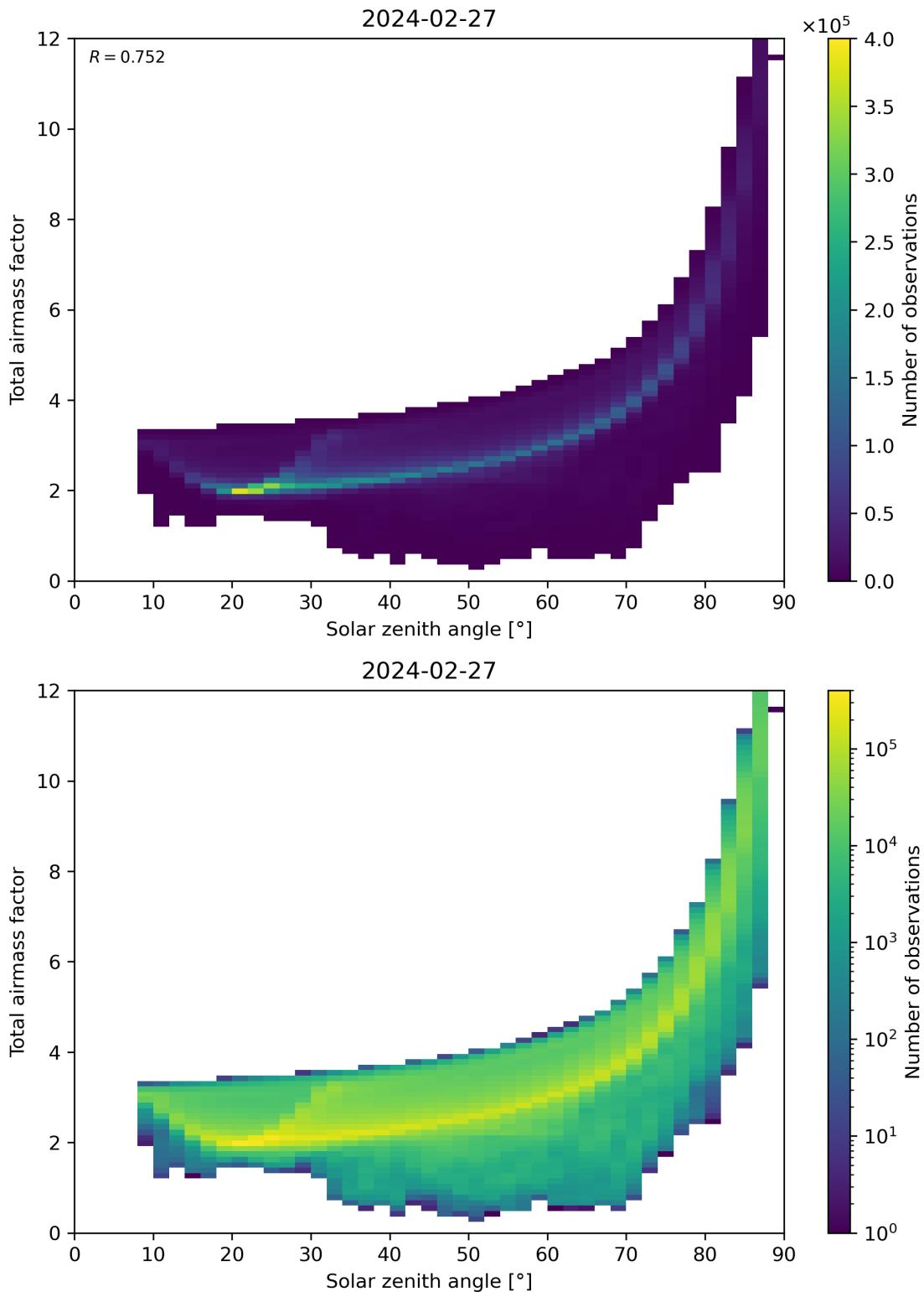
Figure 146: Scatter density plot of “Solar zenith angle” against “Total airmass factor” for 2024-02-27 to 2024-02-28.
