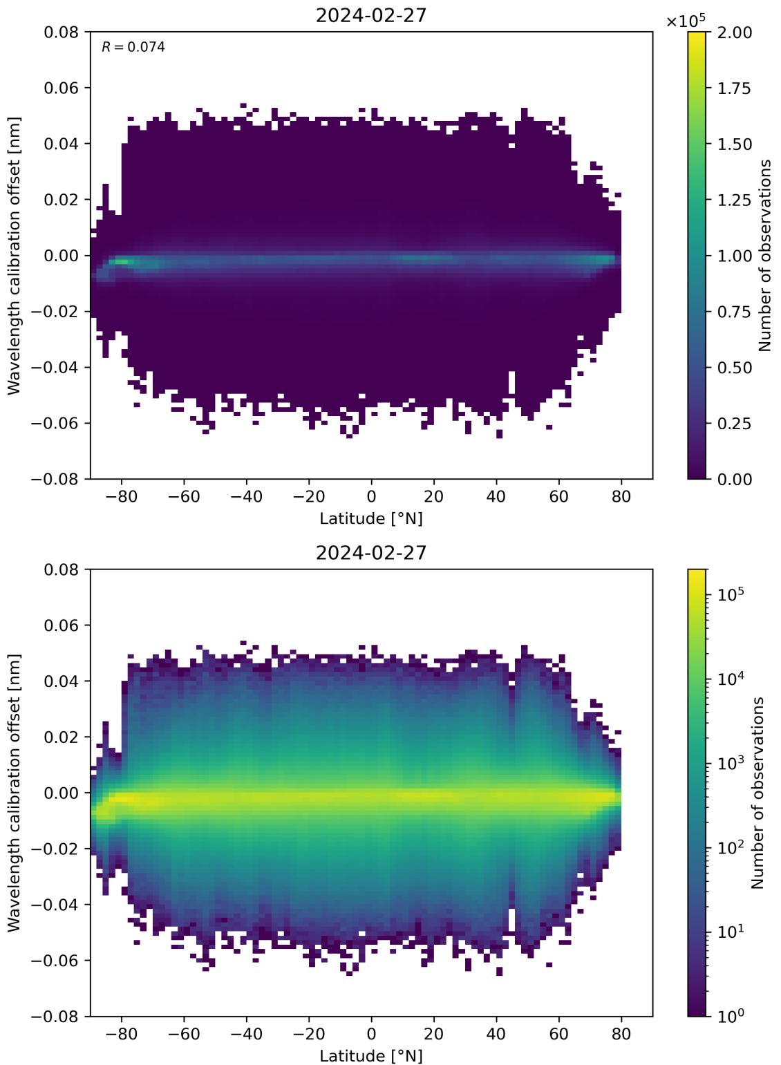
Figure 95: Scatter density plot of “Latitude” against “Wavelength calibration offset” for 2024-02-27 to 2024-02-28.
