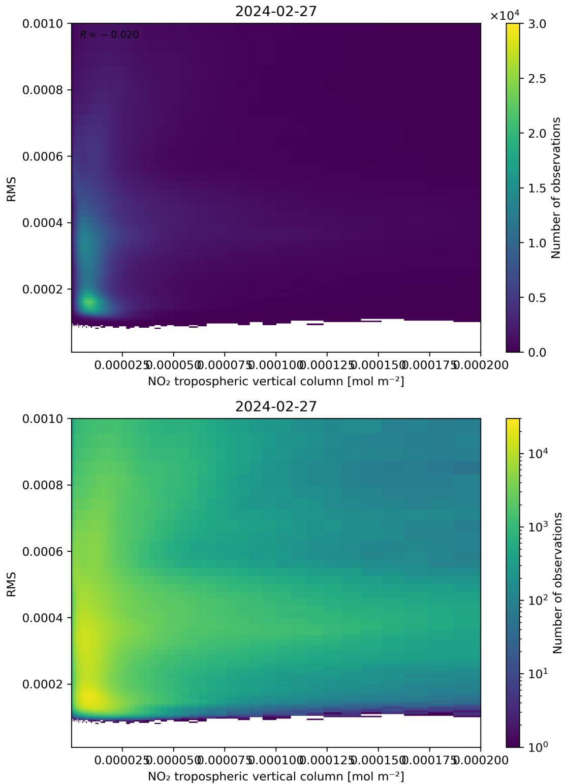
Figure 142: Scatter density plot of “NO<sub>2</sub> tropospheric vertical column” against “RMS” for 2024-02-27 to 2024-02-28.
