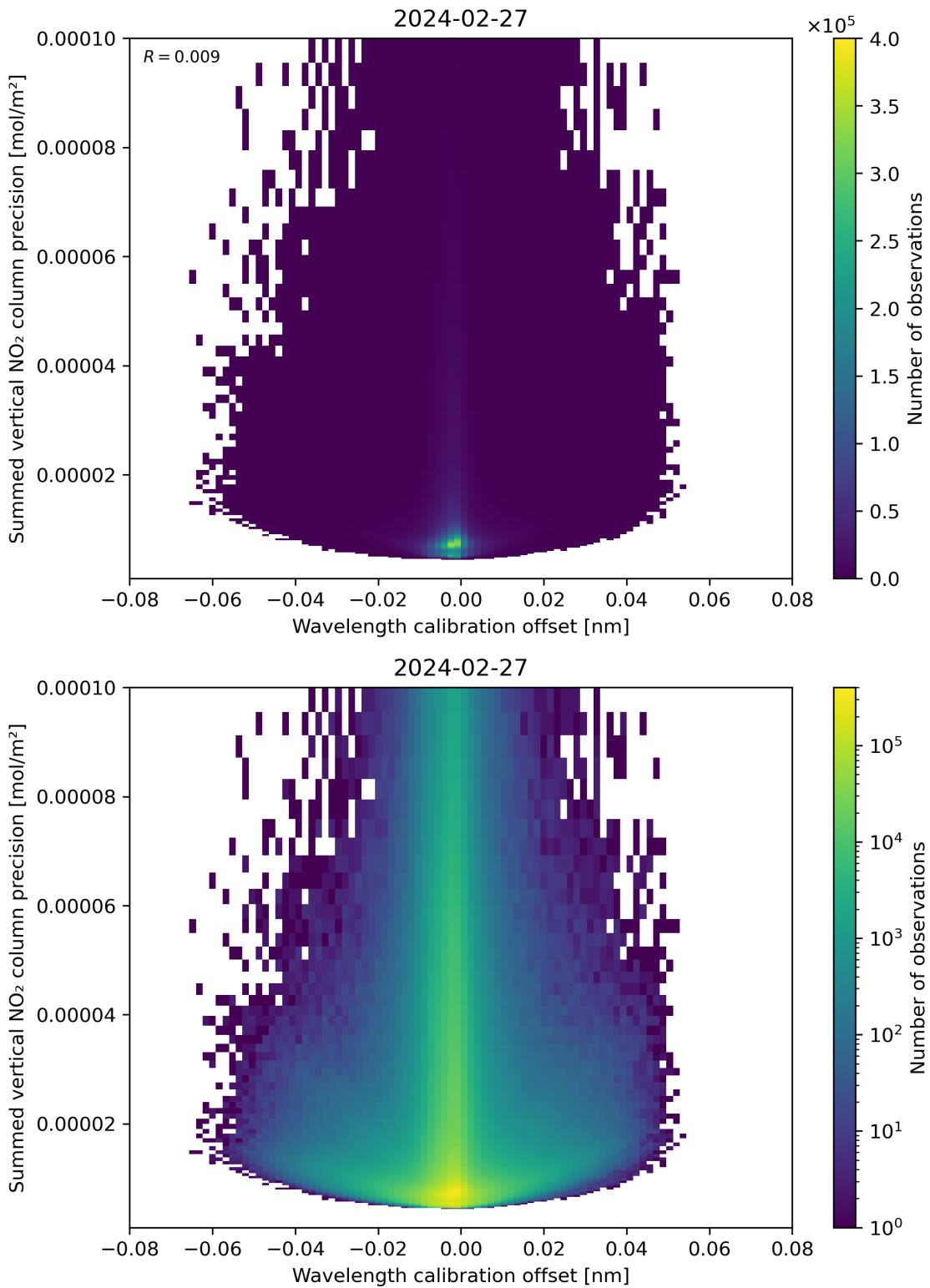
Figure 178: Scatter density plot of “Wavelength calibration offset” against “Summed vertical NO<sub>2</sub> column precision” for 2024-02-27 to 2024-02-28.
