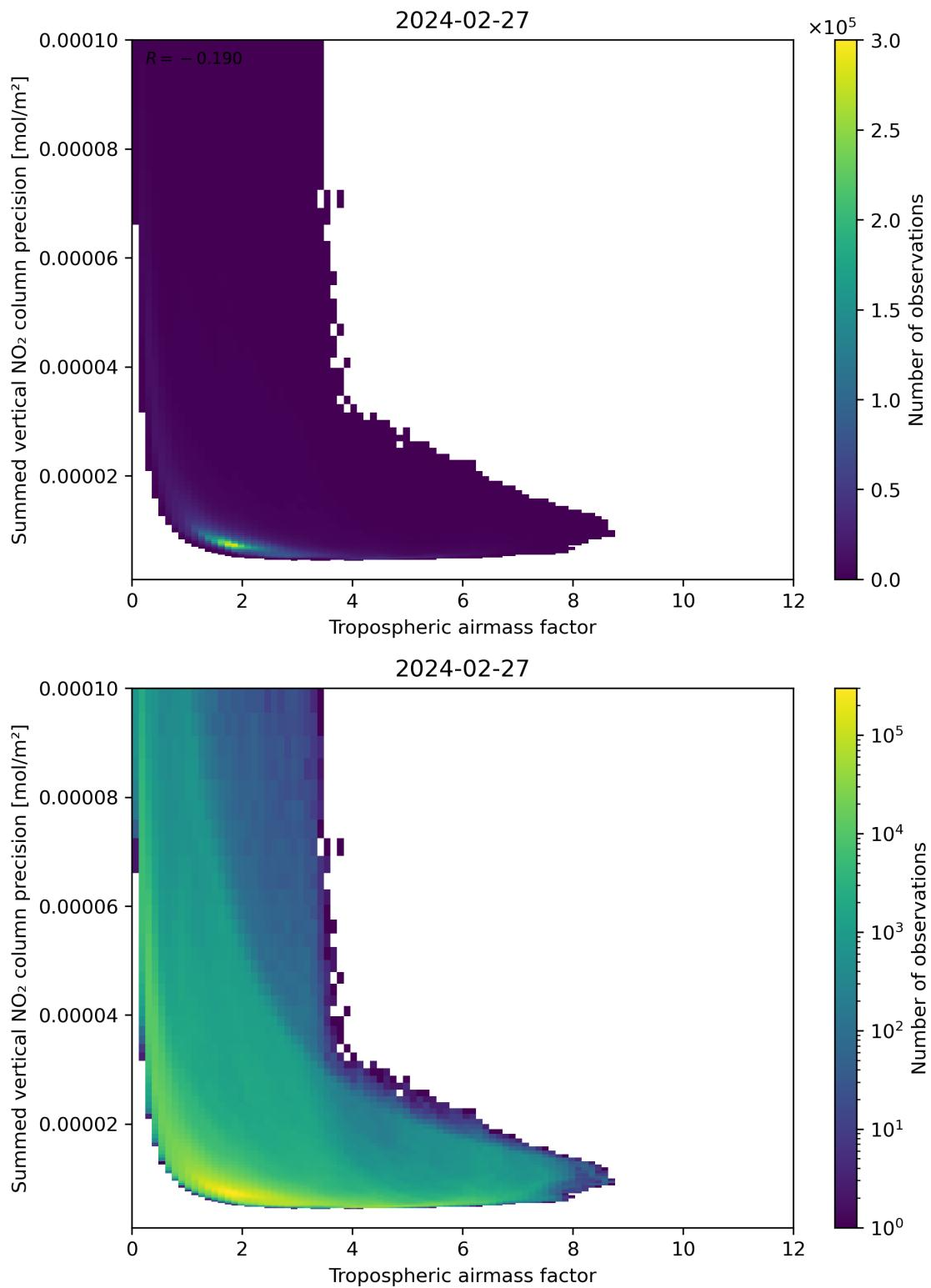
Figure 76: Scatter density plot of “Tropospheric airmass factor” against “Summed vertical NO<sub>2</sub> column precision” for 2024-02-27 to 2024-02-28.
