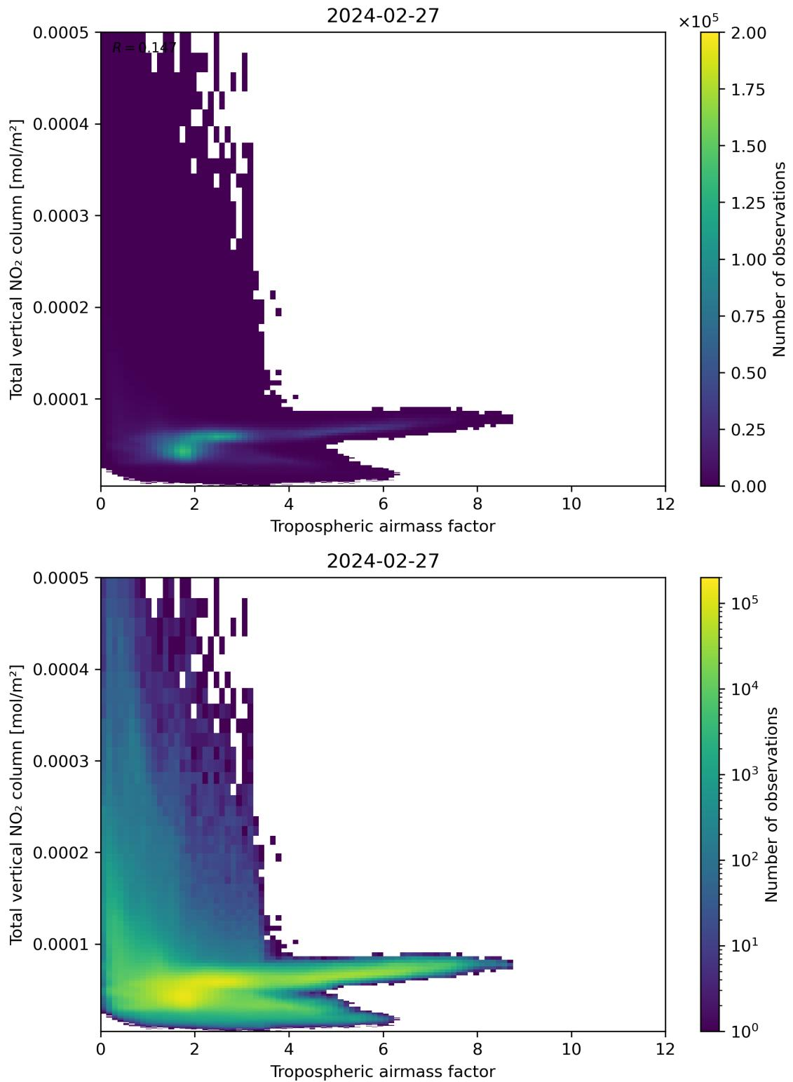
Figure 77: Scatter density plot of “Tropospheric airmass factor” against “Total vertical NO<sub>2</sub> column” for 2024-02-27 to 2024-02-28.
