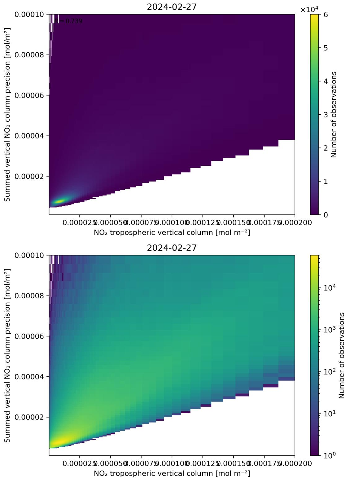
Figure 127: Scatter density plot of “NO<sub>2</sub> tropospheric vertical column” against “Summed vertical NO<sub>2</sub> column precision” for 2024-02-27 to 2024-02-28.
