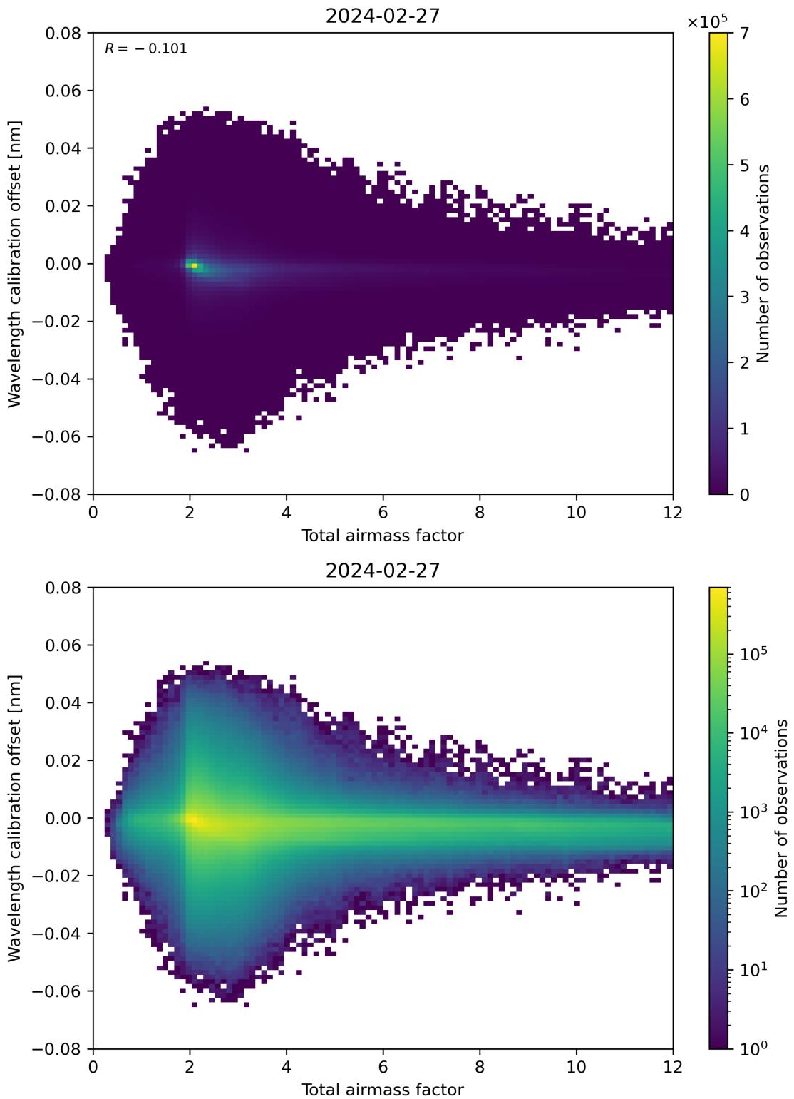
Figure 70: Scatter density plot of “Total airmass factor” against “Wavelength calibration offset” for 2024-02-27 to 2024-02-28.
