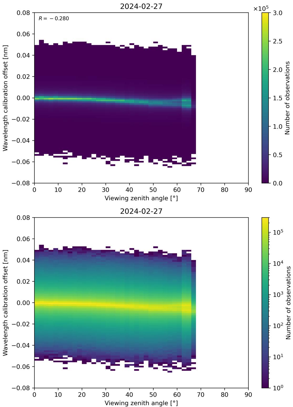
Figure 173: Scatter density plot of “Viewing zenith angle” against “Wavelength calibration offset” for 2024-02-27 to 2024-02-28.
