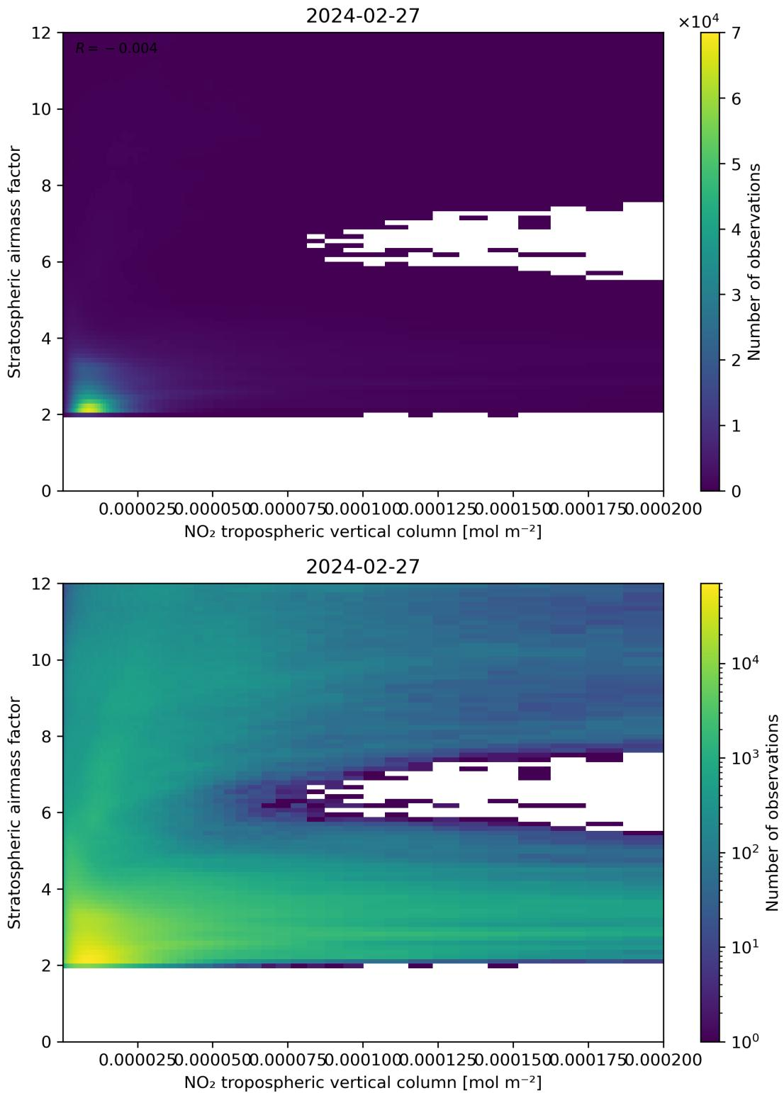
Figure 121: Scatter density plot of “NO<sub>2</sub> tropospheric vertical column” against “Stratospheric airmass factor” for 2024-02-27 to 2024-02-28.
