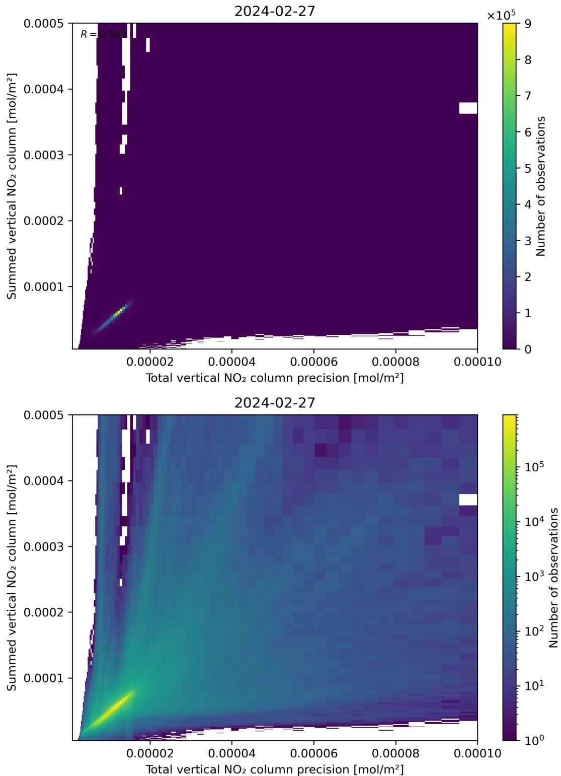
Figure 117: Scatter density plot of “Total vertical NO<sub>2</sub> column precision” against “Summed vertical NO<sub>2</sub> column” for 2024-02-27 to 2024-02-28.
